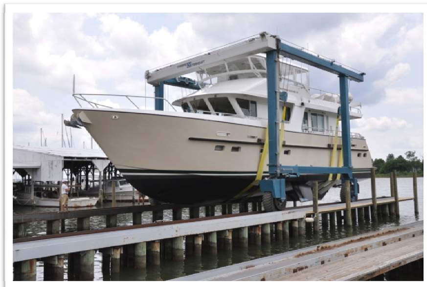
73' Motor Yacht in Deltaville Boatyard's New 75Ton Travel Lift
